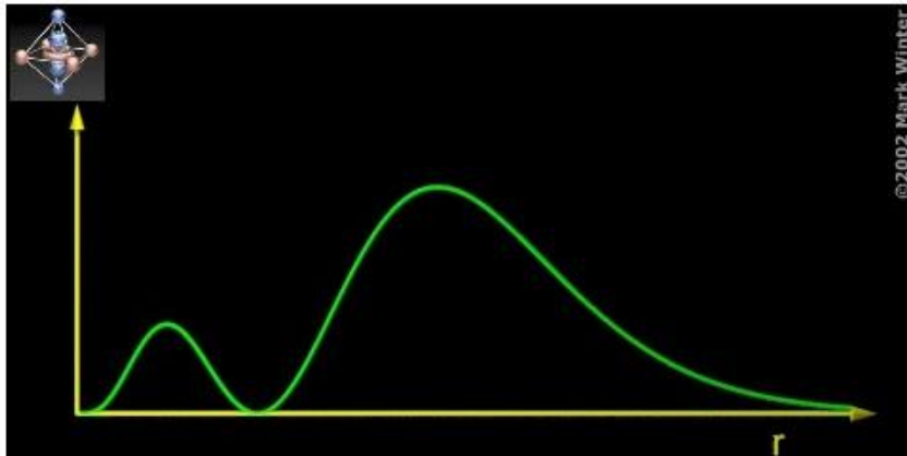
Schematic plot of the 3p radial distribution function r^2R_{3p}^2 ( R_{3p} = radial wave function).
